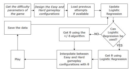
Fig. 1. Flowchart of the  $\delta$ -logit algorithm Steps in italic are design steps that needs to be done manually
